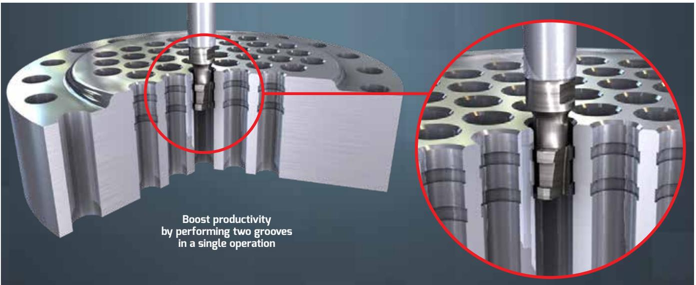
Boost productivity by performing two grooves in a single operation
