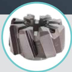
Interchangeable left-hand solid carbide reaming heads (shell reamers) with a quick change bayonet mechanism for H7 hole tolerance high speed reaming of through holes
