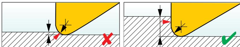
5 Use an insert with an overall positive geometry to reduce the cutting forces:
