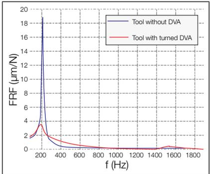
The border between a stable cut and an unstable one can be demonstrated in the plane of depth of cut ( $a_p$ ) and spindle speed and it is known as the Stability Lobe Diagram (SLD). The SLD can be used to find the machining parameters that result in the maximum chatter-free material removal rate. The SLD can be obtained using a tool FRF and machining conditions.
