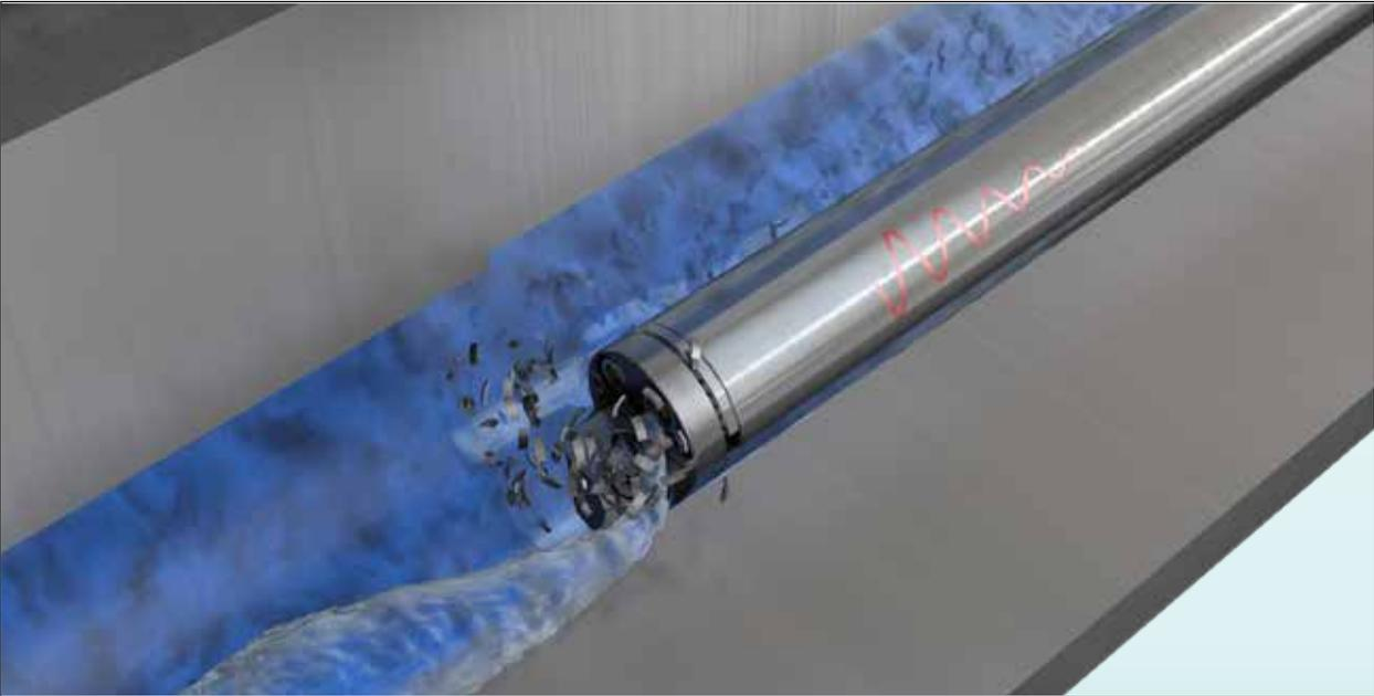
Example: For a bore diameter of 80 mm (3") it is recommended to use a 60 mm (2.5") bar rather than a 80 mm (3") bar. Although the 80 mm bar is stiffer, the lack of space for chip evacuation will decrease the surface finish and can cause breakages.
