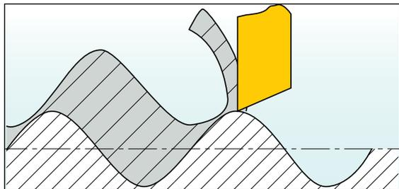
Chatter vibrations are detrimental to the safety and quality of machining operations. They cause a rough surface finish, increase cutting forces, reduce tool and machine life, decrease productivity, and create irritating high noises.
