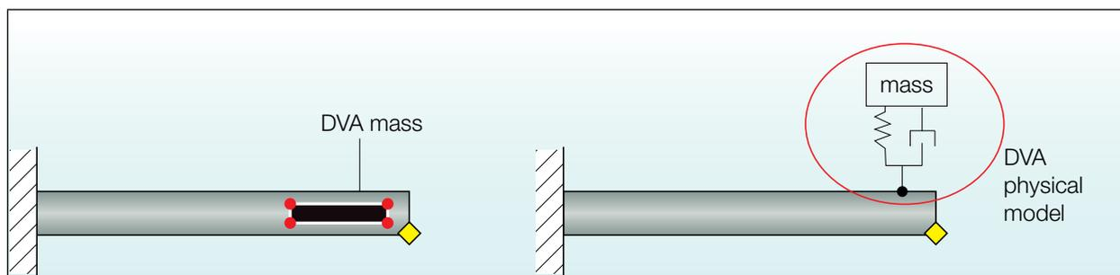
A mechanism is designed to preload the elastomers and therefore to modify the stiffness of their equivalent spring. Modification of the spring stiffness causes a change of the DVA natural frequency. The DVA system is tuned such that its natural frequency is brought close to that of the tool without DVA. This is done in order to introduce a phase shift between the tool and the DVA mass vibration, eventually causing attenuation of the oscillation amplitude of the tool.
